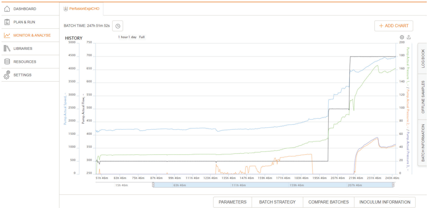
Figure 8. PuraLev Console System PCS-i30SU.1 parameters recorded in eve® during cultivation 1 (pump speed, flow rate, and pressures).
